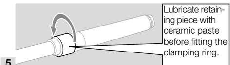
→ Tighten the clamping ring with a torque of 30 Nm.
